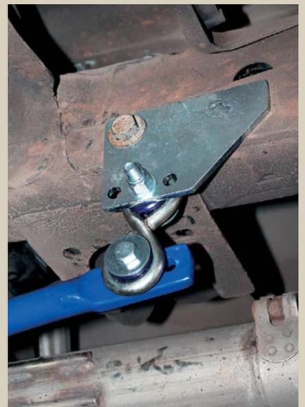
***'The front bar, larger in diameter at 30 mm, is a simple substitution, but of course there is no rear anti-roll bar as standard on the Amarok...'***
